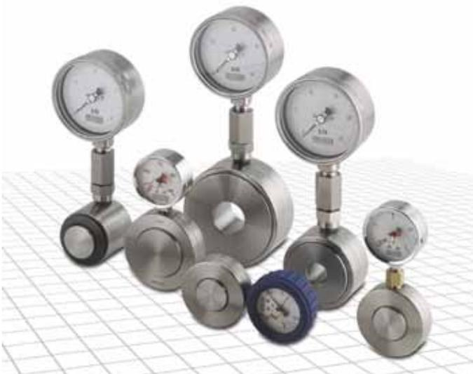
ERICHSEN hydraulic load cells provide a simple and economical method of measuring forces. The technique is based on the hydraulic transmission of forces which act on the piston of the force transducer. This hydraulic pressure is immediately indicated on a display unit with a scale in Newton. Load cells are ideal for maintenance and adjustment work as well as for the use in plants, machines
